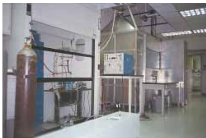
An exposure chamber for respiratory challenge studies. The subject is seated inside the metal chamber and gas or vapour is passed through a laminar flow wall into the chamber, inside which spirometry can be performed
